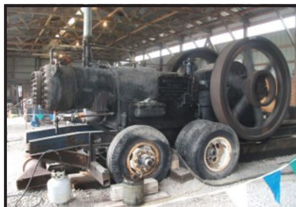
125 HP, 15 Ton Buckeye Engine (one of two running)
